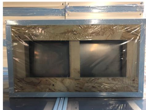
***In the case of 10", 12" or greater walls, the SMART VENT PIP Buck utilizes existing base frames with a 2" extension. Simply apply the 2" extension to the inside face of the window by snapping the extension into the integral snap-in groove. This can be done with a rubber mallet or hand pressure. The extension is available for both standard and custom size units and can be used with all base frames.***
